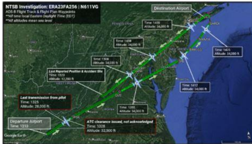
NTSB Figure: Overview of the ADS-B flight track, flight plan waypoints, and select time/altitude labels.
