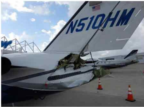
Fig 2 - Mustang Tail Section Damage
